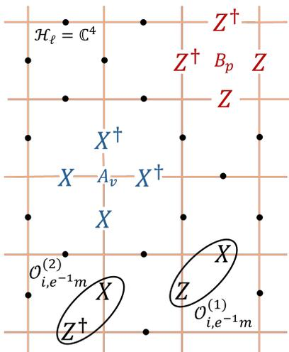
FIG. 2: The  $\mathbb{Z}_4$  Toric code is defined on the 2D square lattice with a  $d = 4$  qudit (black) on each link. The star (plaquette) stabilizers are shown here in blue (red). Short string operators for the  $e^{-1}m$  anyon are also shown.
