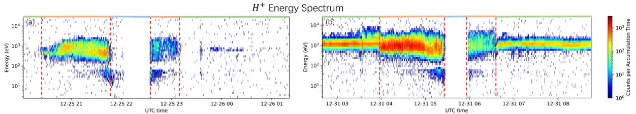
Figure 5:  $H^+$  energy spectrum after noise reduction. The left figure shows the situation when the solar wind signal is weak, while the right figure corresponds to a clear solar wind signal. The red dashed lines and the color bars above the figure have the same meaning as in Fig. 3 (a)
