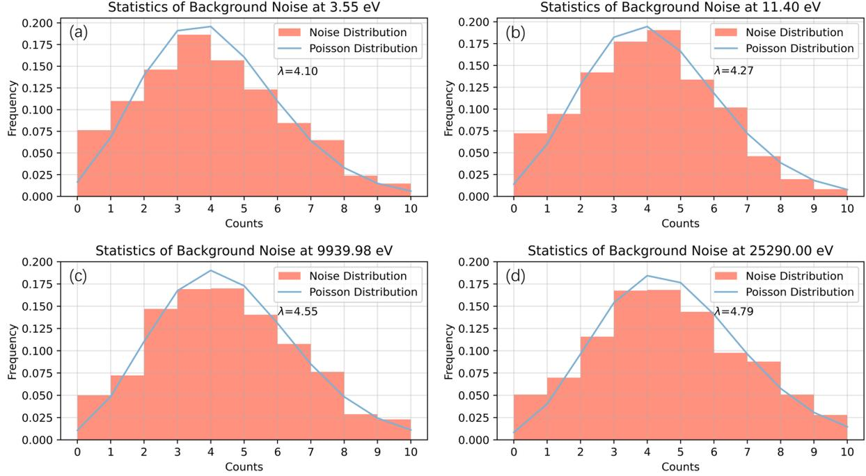
Figure 10: The red histograms denote the statistical distributions of the background noise at different energy channels from December 29 15:00 UT to December 30 18:00 UT, and the blue lines denote the corresponding Poisson distributions with fitted parameters  $\lambda$ , whose values are given in the figure.
