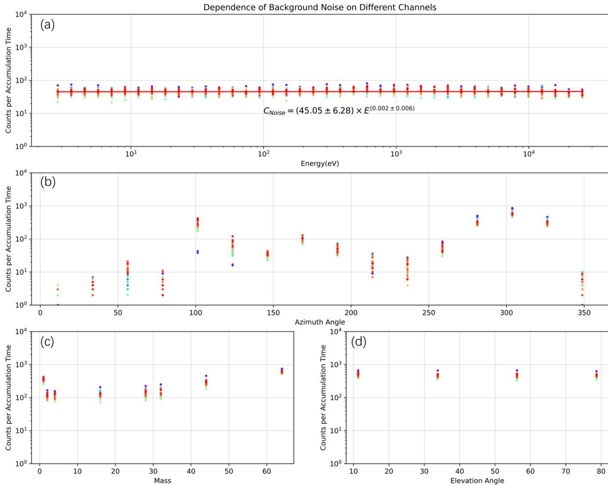
Figure 9: Dependence of the background noise on different channels, including (a) ion energies, (b) azimuth angles, (c) ion masses, (d) elevation angles. Different colors denote different cases that are the same as those in ??.
