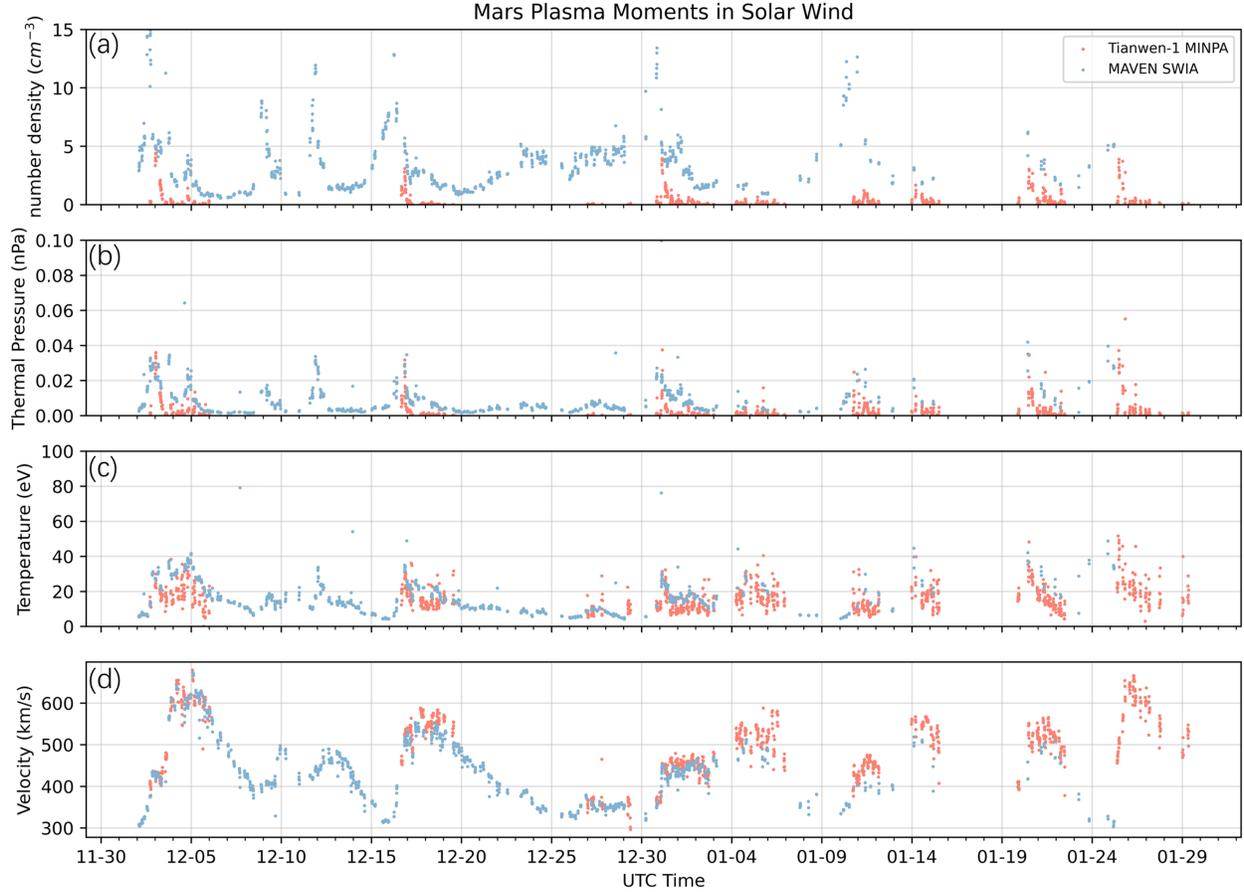
Figure 6: Comparison of the proton plasma moments in the solar wind between Tianwen-1 MINPA (red) and MAVEN SWIA (blue) from December 1, 2021 to January 31, 2022, including number density, velocity, thermal pressure and temperature.
