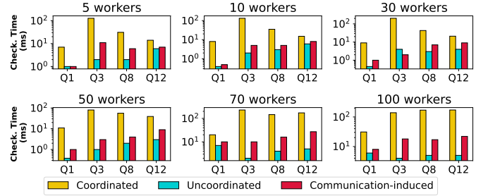
Fig. 8: Average checkpointing time on different parallelisms.
