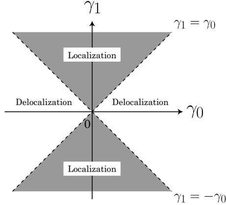
Fig. 2. Phase transition between localization and delocalization. Dot lines are included in delocalization area.
