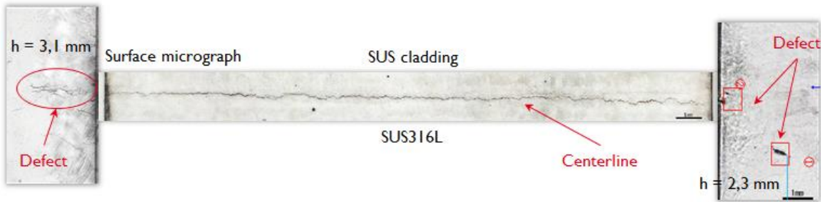
Figure 5 - Micrographs of the inner surface and the two sides of the specimen.
