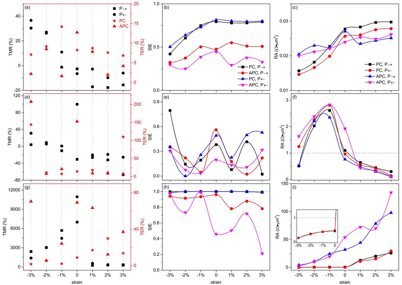
FIG. 6. The TMR [(a), (d), and (g)], SIE [(b), (e) and (h)], and RA [(c), (f), and (i)] as functions of in-plane biaxial strain. Strain effect in the equilibrium state of (a)-(c) Ag-VS<sub>2</sub>-Au MFTJ; (d)-(f) 1T-MoS<sub>2</sub>-VS<sub>2</sub>-2H-PtTe<sub>2</sub> MFTJ; (g)-(i) Fe<sub>3</sub>GaTe<sub>2</sub>-VS<sub>2</sub>-Fe<sub>3</sub>GeTe<sub>2</sub> MFTJ.
