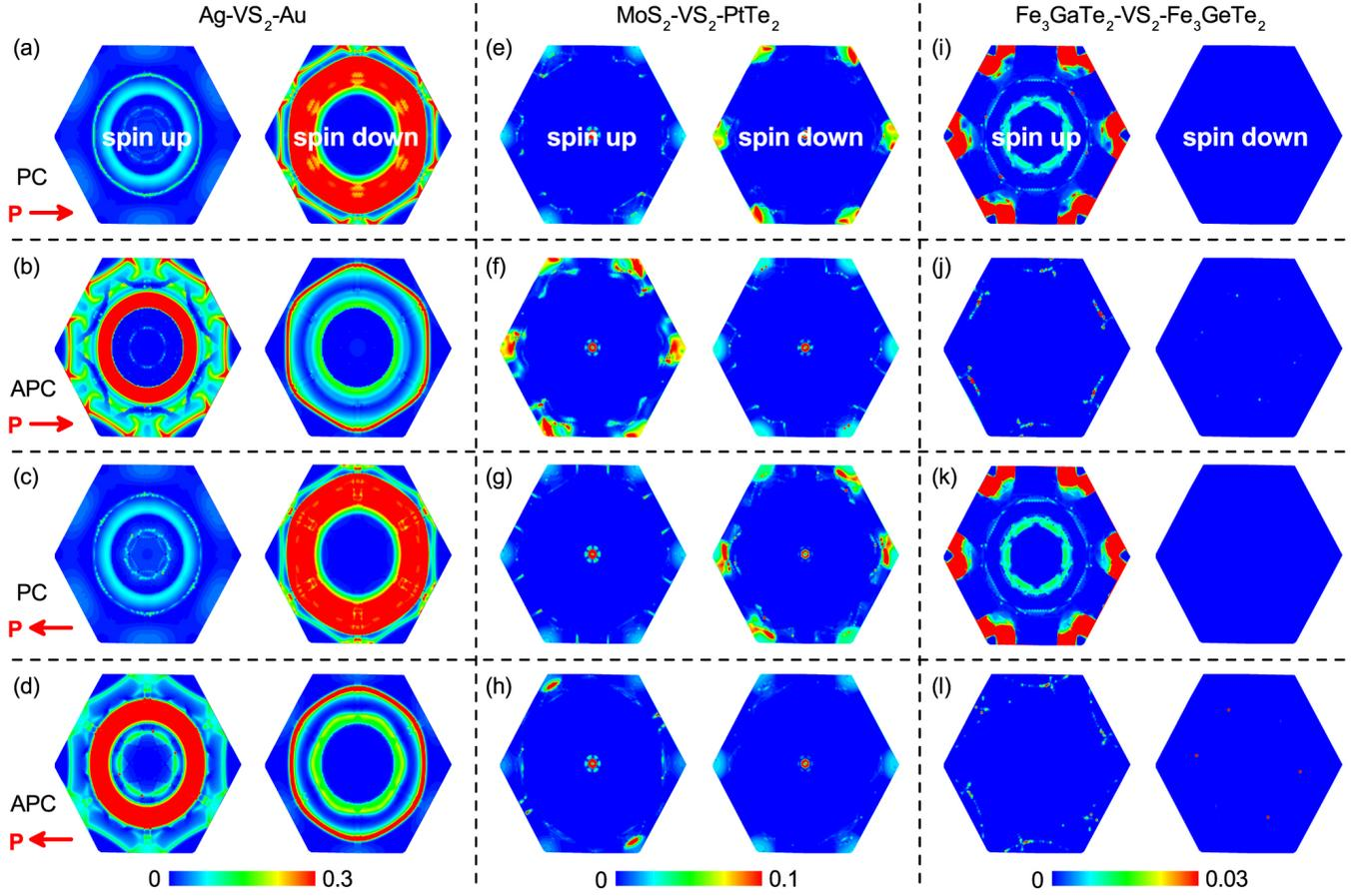
FIG. 5. The  $k_{\parallel}$ -resolved transmission coefficients across the three different  $\text{VS}_2$ -based MFTJs in the 2D Brillouin zone for  $\text{P}\rightarrow/\text{P}\leftarrow$  and  $\text{PC}(\text{M}\uparrow\uparrow)/\text{APC}(\text{M}\uparrow\downarrow)$  states at the Fermi level. (a)-(d)  $\text{Ag-VS}_2\text{-Au}$  MFTJ (e)-(h)  $1\text{T-MoS}_2\text{-VS}_2\text{-2H-PtTe}_2$  MFTJ (i)-(l)  $\text{Fe}_3\text{GaTe}_2\text{-VS}_2\text{-Fe}_3\text{GeTe}_2$  MFTJ.
