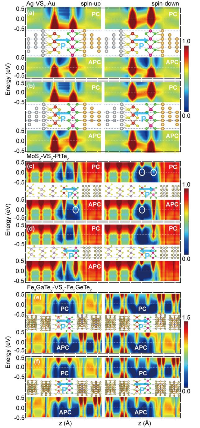
FIG. 4. Spin-resolved PDOS and the corresponding crystal structure of the central scattering region along the transport direction *z*-axis for intrinsic MFTJs with three different types of electrodes in the equilibrium state. White dashed lines mark the Fermi level. The white ovals in panels (c) and (d) mark the minority-state electron density.
