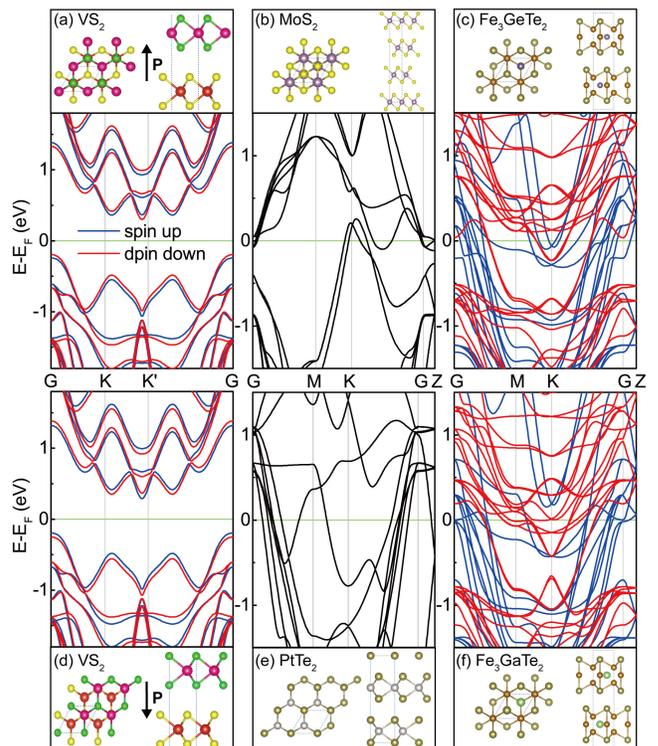
FIG. 2. The Crystal structures and corresponding electronic band structures of (a) and (d) bilayer  $VS_2$  with different ferroelectric polarizations, (b)/(e) bulk  $1T\text{-MoS}_2/2H\text{-PtTe}_2$ , (c)/(f) bulk  $Fe_3GeTe_2/Fe_3GaTe_2$ .
