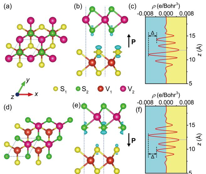
FIG. 1. (a), (d) Top and (b), (e) side views of bilayer  $VS_2$  crystal structures and the difference charge density for opposite out-of-plane ferroelectric polarization. The plane-averaged difference charge density along the  $z$  direction of bilayer  $VS_2$  with different ferroelectric polarization directions. The isosurface value is set to be  $0.00025 \text{ e/Bohr}^3$ . Yellow and blue colors denote charge accumulation and depletion.
