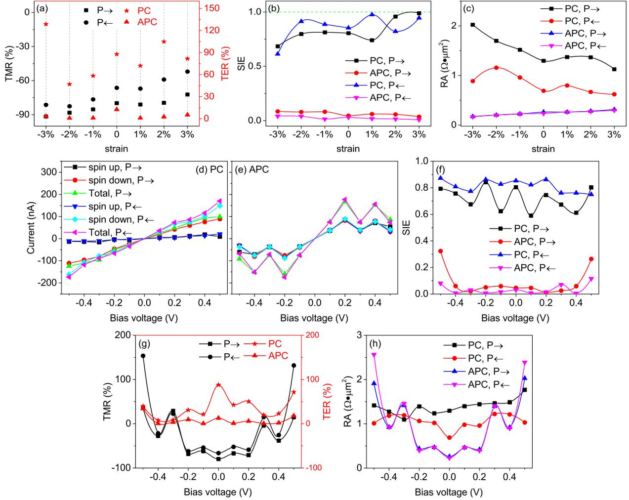
FIG. 9. The TMR (a), SIE (b), and RA (c) as functions of in-plane biaxial strain for Ag-Gra-VS<sub>2</sub>-Gra-Au MFTJ in the equilibrium state. The variation of the current [(d), (e)], spin injection efficiency (SIE) (f), TMR and TER ratios (g), and RA (h) as a function of the bias voltages for Ag-Gra-VS<sub>2</sub>-Gra-Au MFTJ in the non-equilibrium state.
