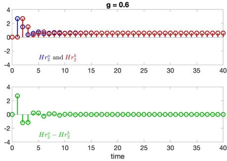
Fig. 3. Respective responses  $Hr_2^a$  and  $Hr_2^b$  to deterministic step signals  $r_2^a$  and  $r_2^b$  when the gain is  $g = 0.6$ . The circle criterion guarantees finite incremental gain and hence the difference  $Hr_2^a - Hr_2^b \in \ell_2$ .
