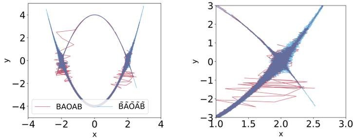
FIG. 12. Plots of the trajectories with the classic underdamped system and the transformed underdamped system. The stepsize is  $h = 0.025$ , rescaled by the average value of the monitor function 0.741 for the classic underdamped. The transformed system is able to visit the upper narrow channel while the classic system can not.
