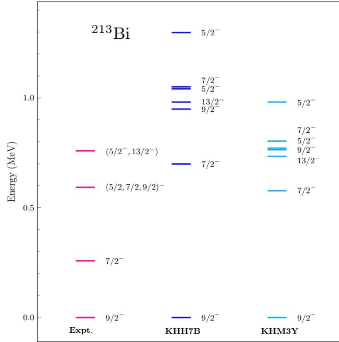
**Figure 11.** Comparison between the theoretical and experimental [51] energy levels in  $^{213}\text{Bi}$  isotope.
