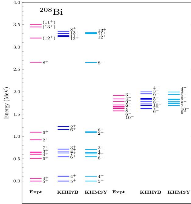
**Figure 4.** Comparison between the theoretical and experimental [51] energy levels in  $^{208}\text{Bi}$  isotope.
