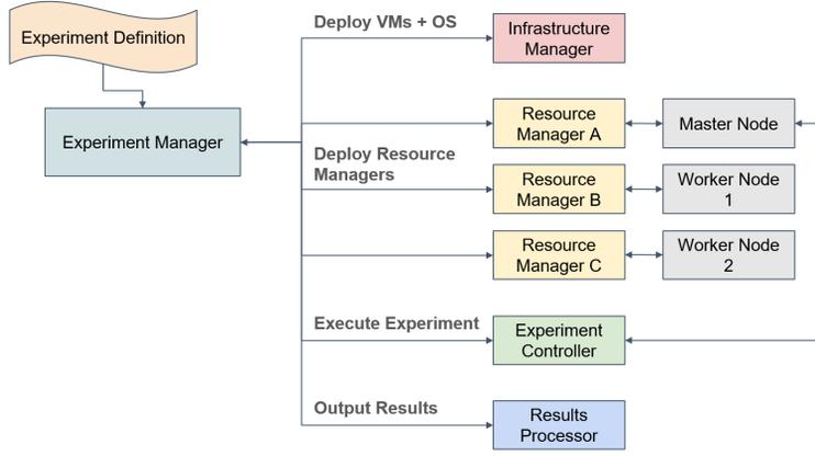
Fig. 2: Main architectural components and interactions.
