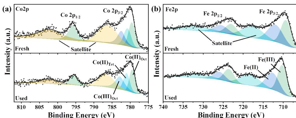
**Fig. 6.** Co 2p (a) and Fe 2p (b) XPS spectra of the fresh and used CoFe<sub>2</sub>O<sub>4</sub>@PC.
