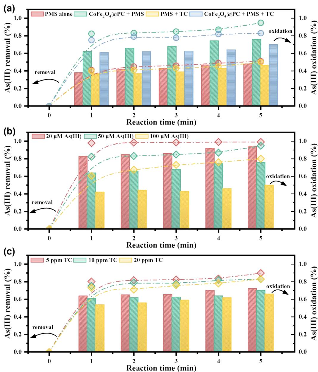
**Fig. 4.** As(III) removal efficiency and oxidation efficiency with different reaction systems ((a) and (d)), different As(III) concentrations ((b) and (e)), and different TC
