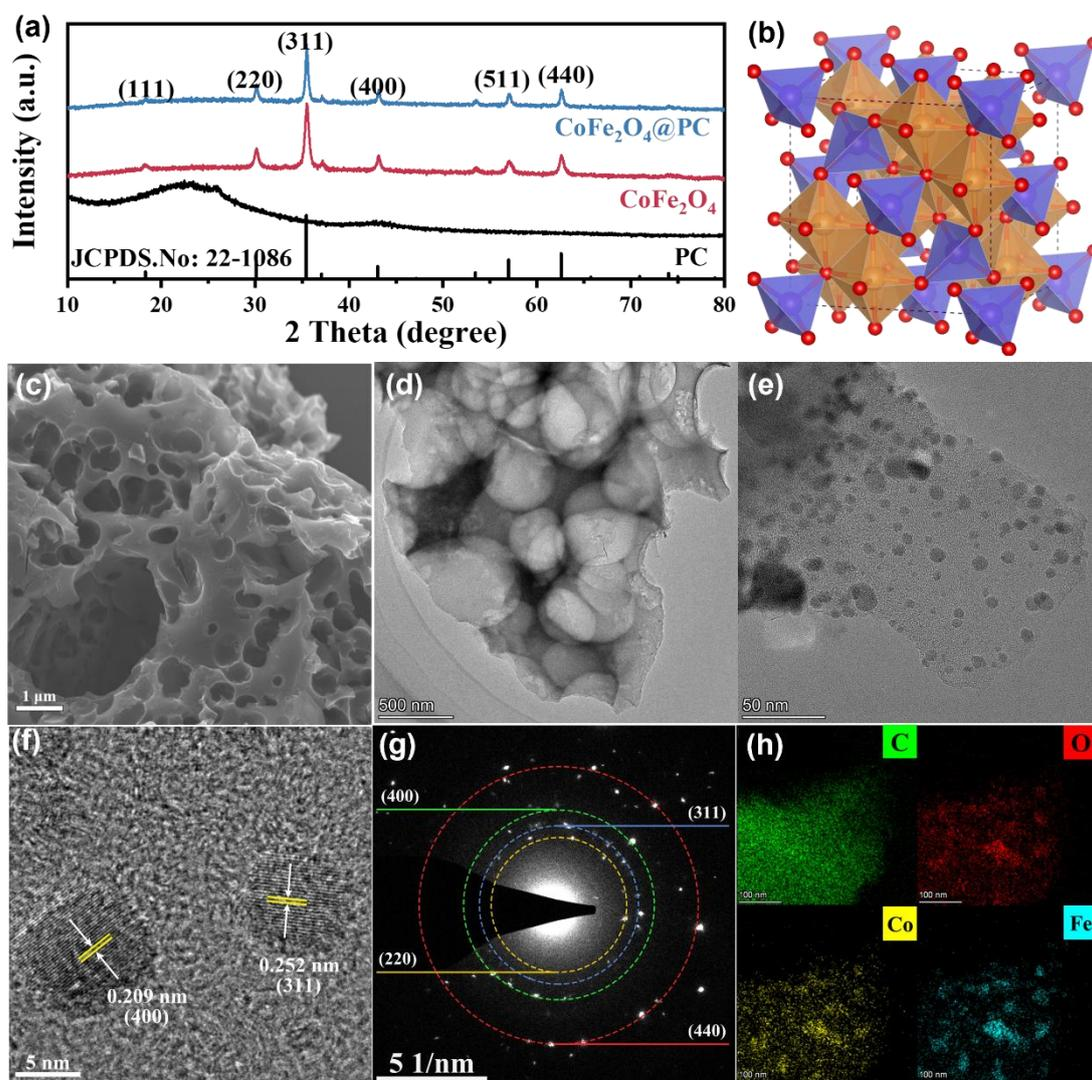
**Fig. 1.** Characterization of prepared catalysts. XRD pattern of PC,  $\text{CoFe}_2\text{O}_4$ , and  $\text{CoFe}_2\text{O}_4@\text{PC}$  (a); Crystal structure of  $\text{CoFe}_2\text{O}_4$  (b); SEM image (c) and TEM image (d); HRTEM image (f); SAED pattern (g); and EDS elemental mapping (h) of  $\text{CoFe}_2\text{O}_4@\text{PC}$ .
