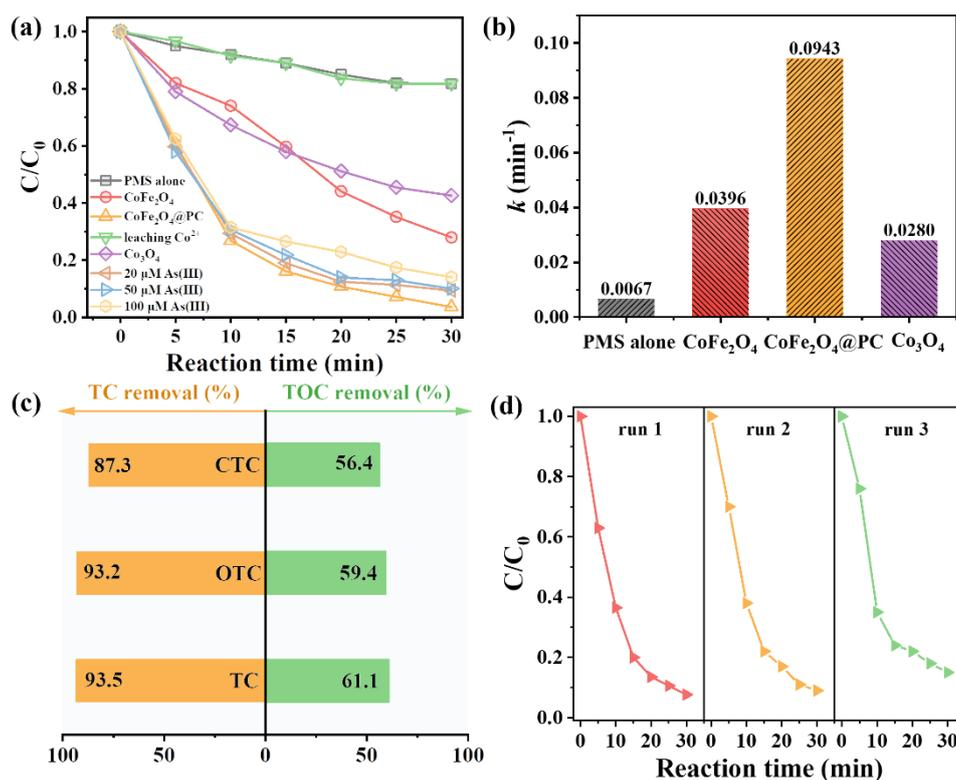
**Fig. 2.** TC removal in various PMS activation systems (a) and corresponding kinetic constant (b); Degradation and mineralization efficiency of TC, CTC, and OTC (c); cycle tests for  $\text{CoFe}_2\text{O}_4@\text{PC}$  (d). Experimental conditions:  $[\text{TC}] = [\text{CTC}] = [\text{OTC}] = 10 \text{ mg/L}$ ,  $[\text{PMS}] = 0.8 \text{ mM}$ ,  $[\text{Catalysts}] = 0.1 \text{ g/L}$ , initial  $\text{pH} = 7$ .
