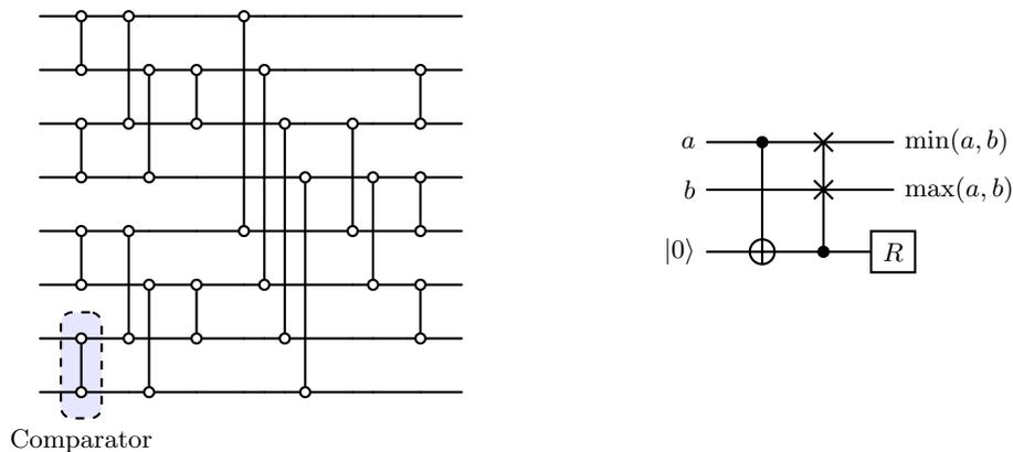
FIG. 6. **Left:** An optimal sorting network for 8 inputs is depicted using 19 comparators with a circuit depth of 6 [89]. **Right:** The 2-input comparator gadget (boxed in the left circuit) is shown, which sorts the binary inputs  $a, b$  using an ancilla, a CNOT gate and a Fredkin (CSWAP) gate. The Fredkin gate can be decomposed into 7 CNOT gates and single-qubit rotations [90].
