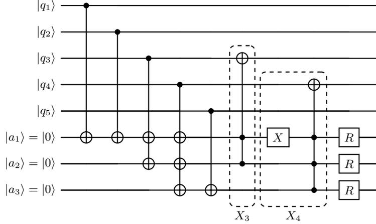
FIG. 5. Two examples of how to implement dynamics in (D5). There are three stabilizers:  $S_1 = Z_1Z_2Z_3Z_4$ ,  $S_2 = Z_3Z_4$  and  $S_3 = Z_4Z_5$  so we need three ancilla qubits to extract syndromes by the CNOT gates outside the dashed boxes. The gates in the boxes apply  $X_3$  and  $X_4$  according to different syndromes. The reset channel  $R$  forces ancilla qubits to their initial state  $|0\rangle$ .
