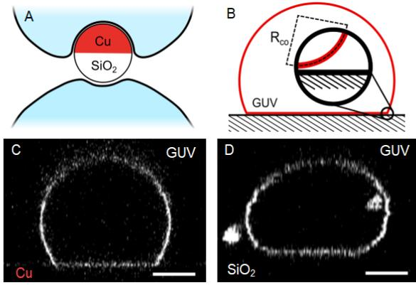
Figure 5. (a) Sketch illustrating the difference of GUV membrane interaction with the copper coated surface and the bare  $\text{SiO}_2$  surface of the Janus particle. (b) Sketch of the experiment and definition of the contact curvature radius  $R_{co}$ . (c) Representative transverse views ( $xz$  plane) from a confocal microscopy acquisitions of osmotically deflated POPC GUVs sedimented on a Copper coated glass substrate and (d) on a bare glass substrate.
