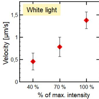
FIG. 1. Average (on  $N=10$  trajectories) measured values for projected velocity  $V$  for different illumination intensities (in percentage of maximum illumination intensity) at 100 mM glucose concentration.
