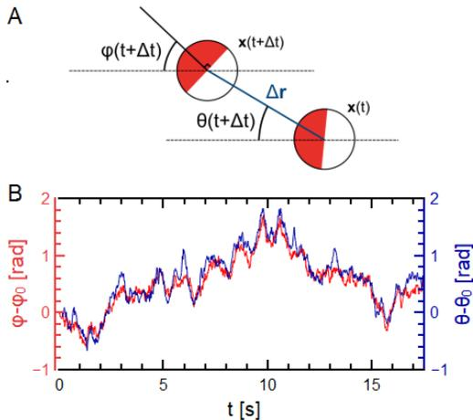
FIG. 5. (a) Sketch defining the orientation  $\phi$  and the direction of motion  $\theta$  of a Janus swimmer. (b) Temporal evolution of  $\phi - \phi_0$  and  $\theta - \theta_0$  where  $\phi_0 = \theta_0 = 0$ . The curve of  $\theta - \theta_0$  was obtained by performing a sliding average over  $N = 20$  points to get rid of the noise arising from short times brownian motion and evidence the direction given by the active propulsion force.
