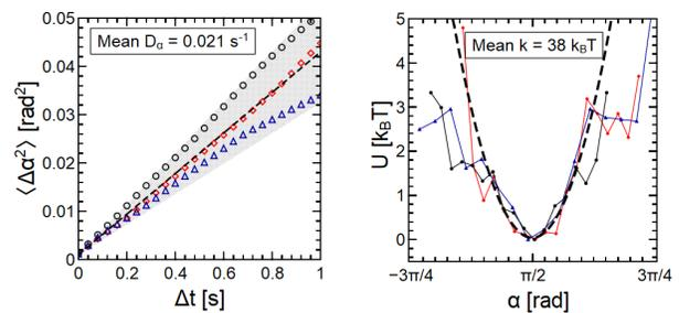
FIG. 8. (a) Mean squared angular displacement curve obtained from the variations of  $L$  for 3 trajectories with associated fits in plain lines. (b) Effective potential  $U$  obtained from position histogram. Black dashed line shows the mean quadratic potential extracted from fits of the 3 potentials, giving the a stiffness value  $k$ .
