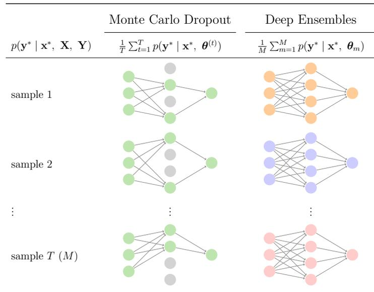
Figure 5: **Overview of uncertainty estimation methods.** Forward passes are generated differently depending on the method. In MC dropout, different units are dropped out from a NN; in Deep Ensembles, multiple independent NNs are used, with different parameter initializations and noise in the SGD training process.
