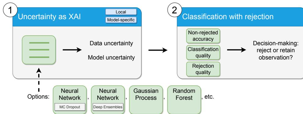
Figure 2: **General uncertainty framework.** The framework consists of two stages: (i) uncertainty estimation as XAI and (ii) classification with rejection. It can be applied to multiple ML models, each having one or more specific uncertainty techniques.
