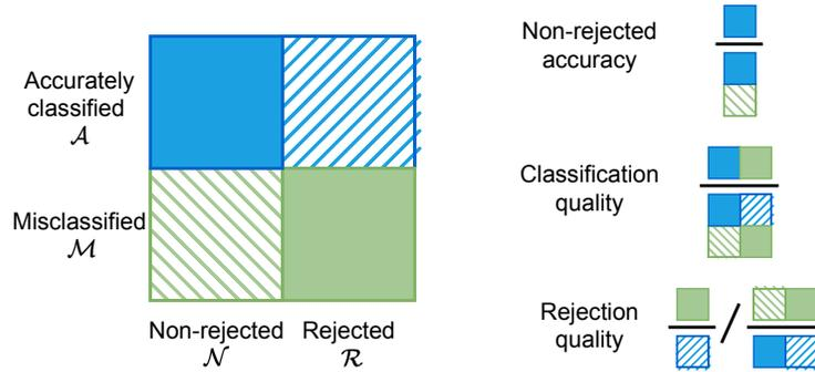
Figure 4: **Performance measures for classification with rejection.** Three performance measures are proposed by Condessa et al. (2017) to find the optimal rejection point. Figure adapted from Mena et al. (2021).
