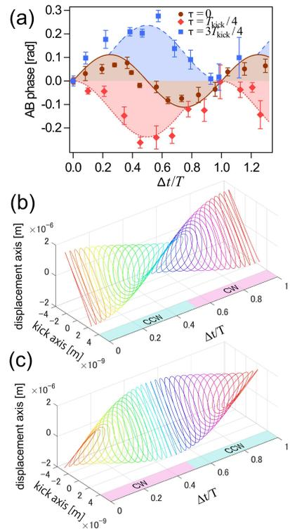
FIG. 2. (a): The time-dependent AB phase at three different delay times  $\tau$ . In panels (b) and (c), the calculated rotational orbits of the ion in the nearly two-dimensional isotropic potential are shown for  $\tau = T_{\text{kick}}/4$  and  $3T_{\text{kick}}/4$ , respectively.
