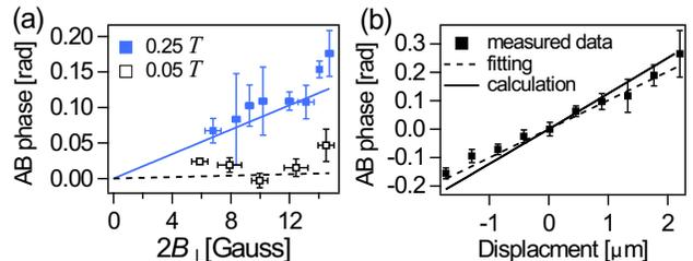
FIG. 3. (a): Magnetic field dependence of the AB phase of ion matter wave interference at delay time  $\tau = T_{\text{kick}}/4$ . (b): Displacement size dependence of the AB phase measured with delay time  $\tau = T$  and displacement time  $\Delta t = T/2$ .
