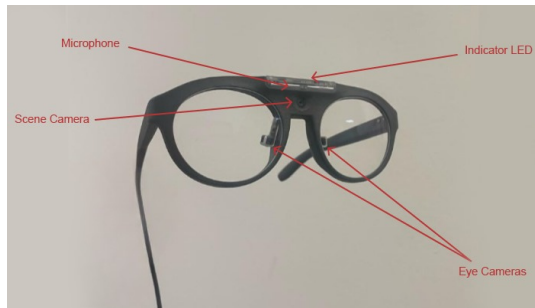
Fig. 2: Pupil labs Neon eye tracker.
