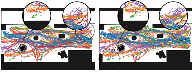
Figure 12. Filtering methods in a 4-minute recording from Scenario 1. Left: trajectories filtered using the most reliable marker. Right: trajectories filtered using the average of the tracking locations of each marker. Although the average tracking markers method provides longer tracks, it induces jerkier trajectories, especially near the boundaries of the motion capture volume (e.g. bottom left and top right).
