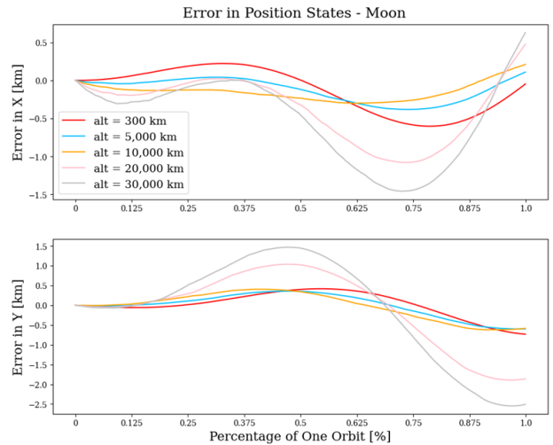
Fig. 7. Error in position states over one orbital period for the Moon.
