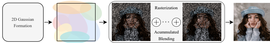
Fig. 2: Our proposed GaussianImage framework. 2D Gaussians are first formatted and then rasterized to generate the output image. The rasterizer uses our proposed accumulated blending for efficient 2D image representation.
