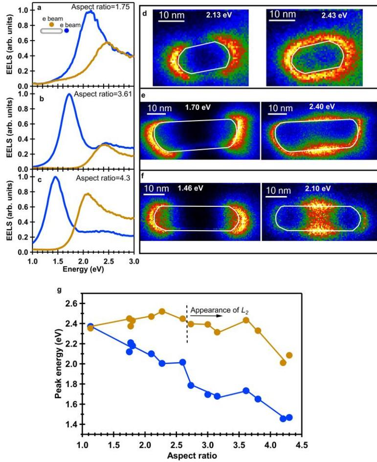
Figure 2: Experimental EEL spectra and EELS maps of gold nanorods of different aspect ratios. (a)-(c) EEL spectra at two different impact parameters: tip (blue spectra) and center (brown spectra). (d)-(f) EELS maps at energies corresponding to peaks of (a)-(c). (g) Evolution of the plasmon peak energy with the rod aspect ratio. The second-order longitudinal mode appears for rod aspect ratios larger than 2.7.
