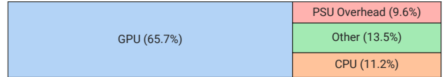
Figure 9: Average power distribution of hardware modules in Seren GPU servers, gathered from IPMI and DCGM.
