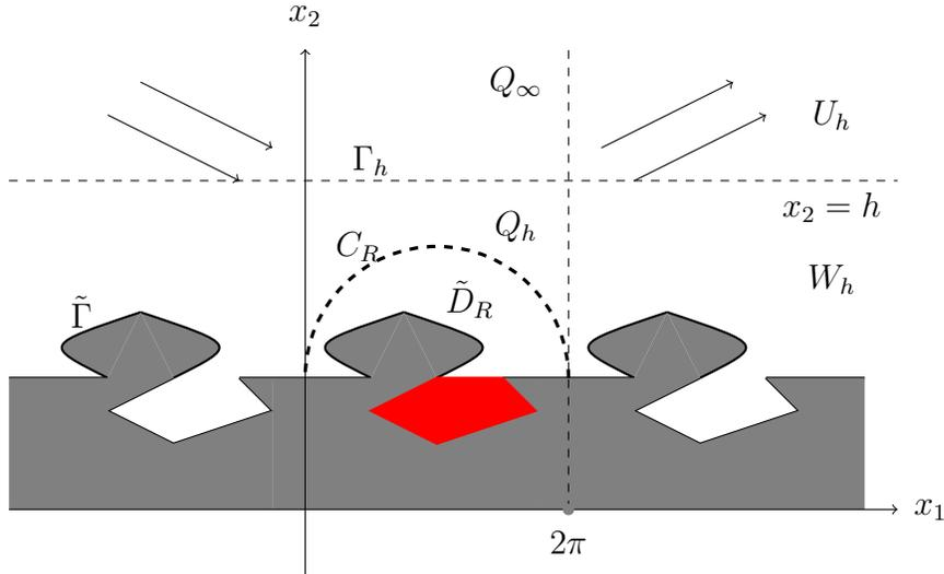
FIGURE 1. Illustration of wave scattering from a perfectly reflecting periodic curve with a local perturbation in  $(0, 2\pi)$ . The red area denotes the perturbed domain. The scattering interface is supposed to be a non-self-intersecting curve.
