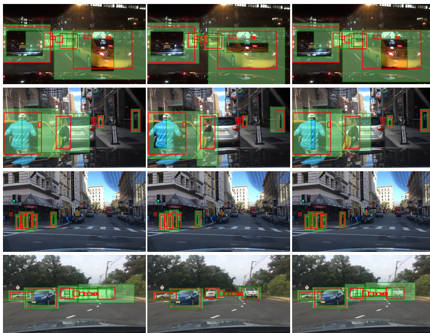
Fig. 14: Examples of conformal bounding box intervals produced by our two-step approach on BDD100k for a mixed set of classes. Left to right by column: using ClassThr in combination with Box-Std, Box-Ens or Box-CQR. True bounding boxes are in red, two-sided prediction interval regions are shaded in green.
