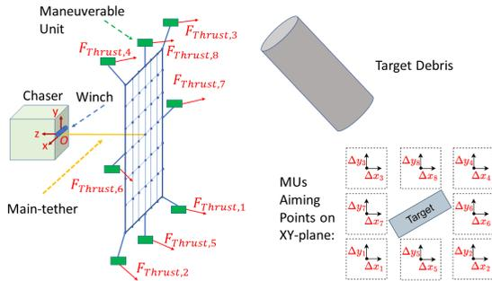
Fig. 1: Representation of the 8-MU Tether-net System
