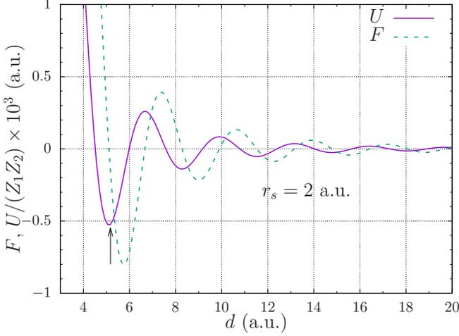
FIG. 1. The potential energy  $U$  (11) and the force  $F$  (10) versus the distance  $d$  between two point charges  $Z_1$  and  $Z_2$  in the HEG of the density parameter  $r_s = 2$  a.u. The equilibrium distance between the charges (marked with an arrow) is  $d = 5.17$  a.u.  $\chi^h(q, 0)$  used was obtained with Eq. (17) and the MCP07 approximation for  $f_{xc}(q, 0)$ . [16]
