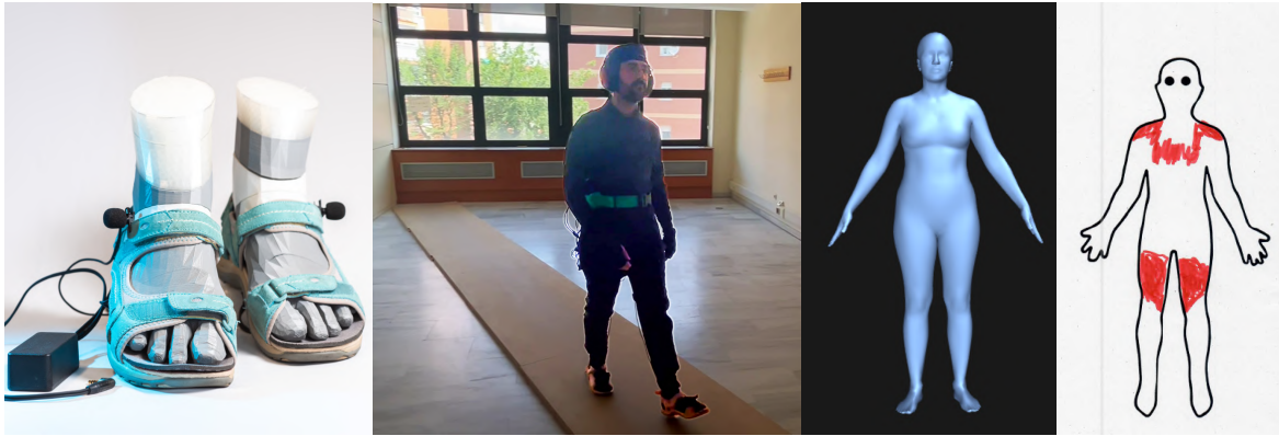
Figure 2: Detail of the microphones in the prototype; laboratory setup and participant wearing prototype and mocap suit; Body Visualizer tool employed to measure visualized body size/weight; an example of a body map filled by participants.
