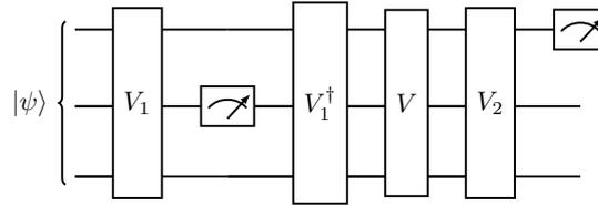
Figure 10: Ancilla-free quantum circuit that evaluates  $\mathcal{R}e[\langle \psi | \hat{V}_2^\dagger \hat{V}_1 | \psi \rangle]$ . The first measurement prepares the state  $\hat{P}_{1,\pm} |\psi\rangle / \|\hat{P}_{1,\pm} |\psi\rangle\|$  and the second measurement estimates  $\langle \hat{\sigma}_2 \rangle$ .
