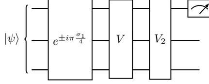
Figure 11: Ancilla-free quantum circuit that evaluates  $\mathcal{Im} [\langle \psi | \hat{V}_2^\dagger \hat{V}_1 | \psi \rangle]$ . Two circuits are required, one with the multi-qubit gate  $e^{i\pi \frac{\hat{\sigma}_1}{4}}$  and the other with  $e^{-i\pi \frac{\hat{\sigma}_1}{4}}$ .
