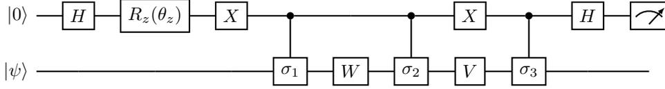
Figure 12: Hadamard test circuit for computing  $\langle \psi | \hat{W}^\dagger \hat{V}^\dagger \hat{\sigma}_3 \hat{V} \hat{\sigma}_2 \hat{W} \hat{\sigma}_1 | \psi \rangle$ . Setting the angle  $\theta_z$  of the  $\hat{R}_z$  gate as 0 or  $-\pi/2$  measures the real and imaginary part, respectively. The value is estimated as  $2P(0) - 1$ , where  $P(0)$  is the probability that the ancilla qubit is measured to be 0.
