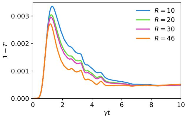
Figure 3: Infidelity between the variational and exact quantum states, computed with Ansatz I with 10 layers and rank  $R = \{10, 20, 30, 46\}$ .
