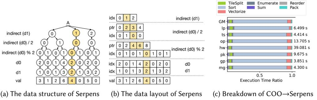
Fig. 12. The Serpens format of the matrix  $A$  in Figure 1a.
