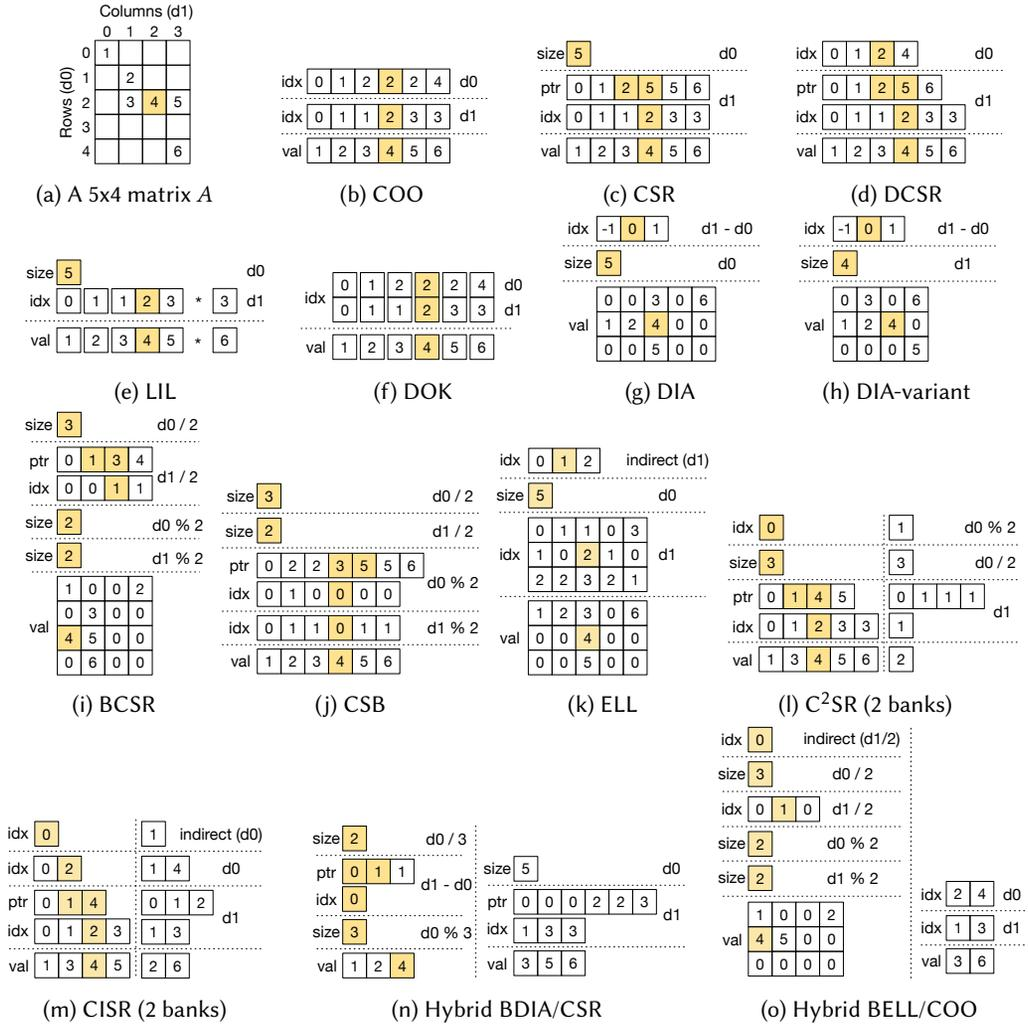
Fig. 1. Different formats of a sparse matrix ( $A$ ) — Yellow-shaded blocks refer to the data structure of the same tensor element. The *size*, *ptr*, *idx*, and *val* labels on the left indicate the size of a dimension, a pointer array, an index array, or a value array. The index expressions on the right denote the index map at each level. Horizontal dotted lines separate different tensor dimensions, while vertical dotted lines divide the matrix  $A$  into sub-matrices.
