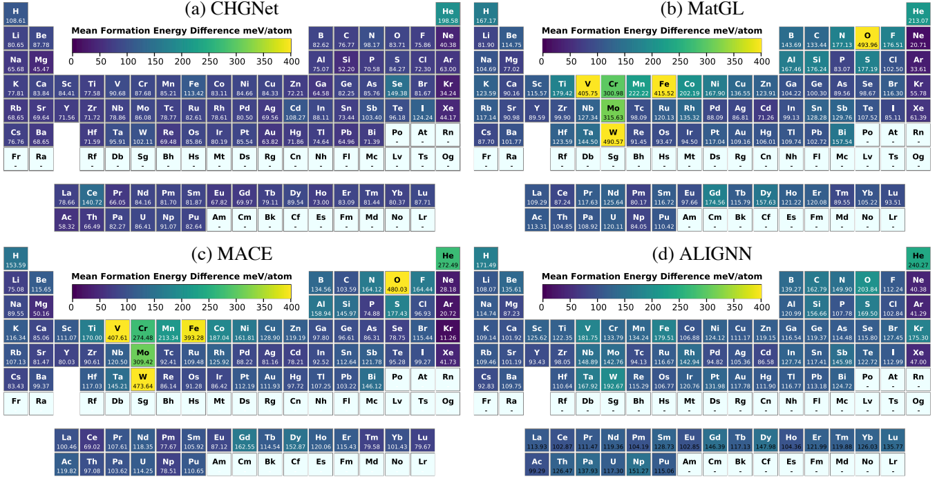
FIGURE 5 Heatmaps of the periodic table for the absolute values of \Delta E_{\text{form}} for the one-shot calculations from the different uMLIPs: (a) CHGNet, (b) MatGL, (c) MACE, and (d) ALIGNN. The figure has been produced with the pymatviz tool 49 .
