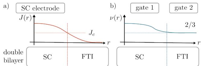
FIG. 7. Realization of a superconductor-to-FTI interface in the bulk of the  $(\theta, 0, -\theta)$  tTMD bilayer using (a) proximity induced superconductivity, and (b) electrostatic gating to tune the density in presence of an intrinsic pairing in the double bilayer.
