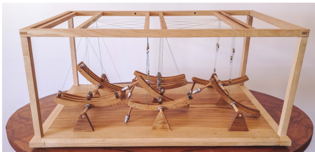
Fig. 6. The mechanical neural network (MNN) is a physical model of an AI model and makes all components of AI literally tangible (Schaffland and Schöning 2023).
