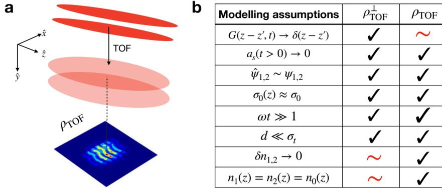
Figure 1: (a) The setup schematics for relative phase measurement of parallel (quasi-)one dimensional Bose gases (red) after time of flight (TOF) adapted from Ref. [26] (b) Comparison table for the assumptions used to derive different models for TOF density [Eqs. (4)-(5)]. The  $\sim$  symbol means that the assumption can be relaxed in general.
