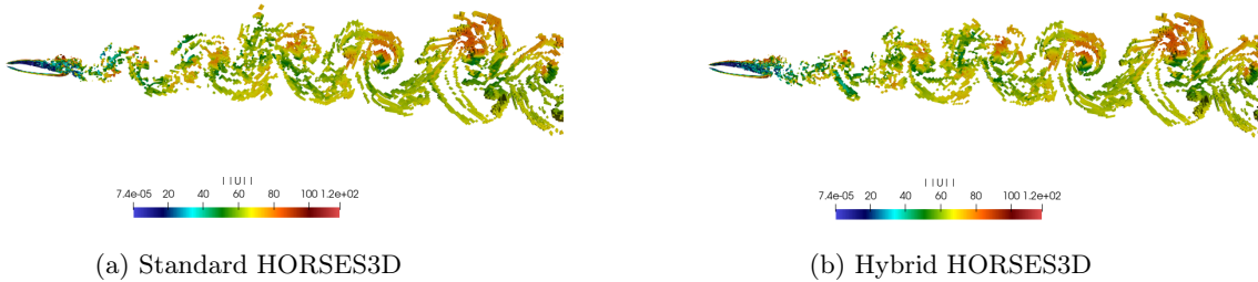
Figure 6: Q -criterion contours, colored with L2 norm of velocity field \|U\|_2 for the flow around an airfoil NACA0012 at Re = 10^4 , \alpha = 10^\circ
