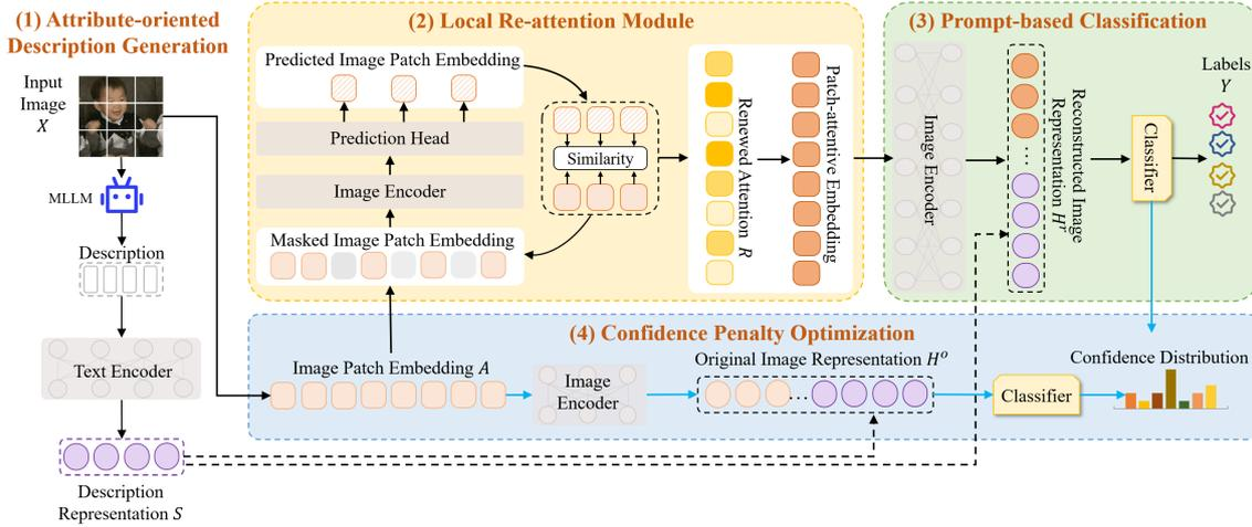
Figure 4: Illustration of the proposed Att<sup>2</sup>PL method comprising (1) Attribute-oriented Description Generation, (2) Local Re-attention Module, (3) Prompt-based Classification, and (4) Confidence Penalty Optimization (blue lines).
