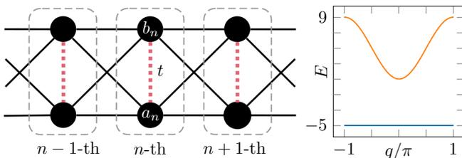
FIG. 1. Left: Schematic of the 1D cross-stitch lattice with two sites per unit cell. The vertical hopping is marked by red dashed lines. Right: The corresponding band structure for the vertical hopping  $t = -5$ .
