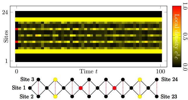
FIG. 5. The time evolution of the initial wavefunction with four hard-core bosons on the 1D diamond lattice is plotted. Here, we set  $t = -5$ . At time zero, two CLSs are located at the second and the seventh unit cells (yellow) with two hard-core bosons positioned at the 10th and the 16th sites (red). The CLSs are fixed as time evolves and two hard-core bosons are strictly confined.
