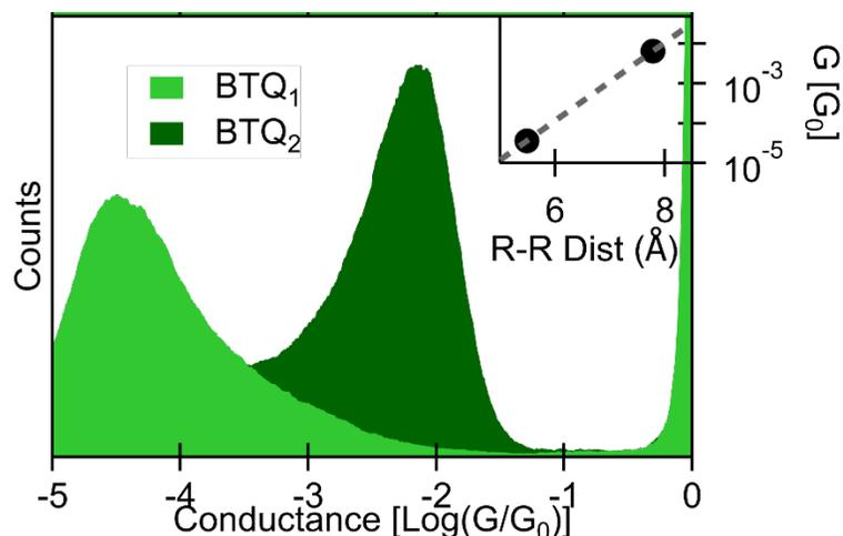
**Fig. 6 | Engineering enhancement in anti-ohmic conductance through synthetic control.** Single-molecule conductance histograms of BTQ<sub>1-2</sub> (structures shown in Fig. 1a) in BNP at  $-500$  mV. Inset: most likely conductance of BTQ<sub>1-2</sub> determined from the histograms plotted against radical-radical (R-R) distance results shows inverse decay and a  $\beta$  value of  $-2.3/\text{\AA}$ .
