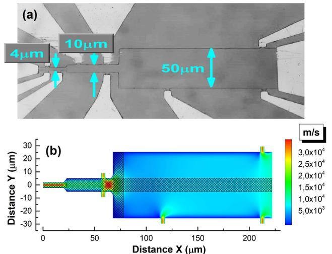
FIG. 2: (Color online) The sample image (a) and the velocity flow contour plot in a variable width hydrodynamic channel calculated with the fluid parameters defined in the text (b). The scanning bands parallel and perpendicular to the channel, determined by the spatial resolution of the PL, are shown as mesh strips.
