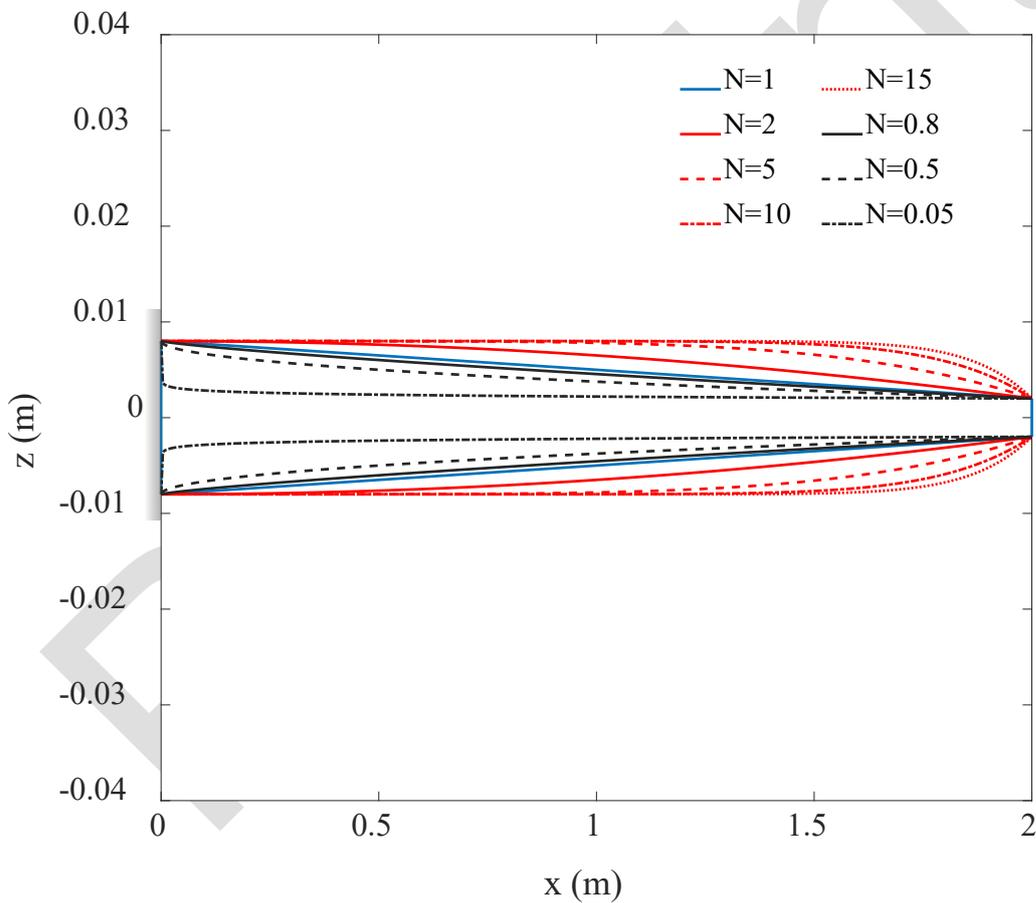
Figure 13. The side view of the tapered beam for different values of gradient index ( $N$ )
