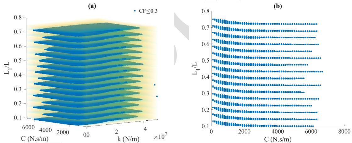
Figure 8. The CF plots stack for the uniform homogenous beam where absorber's location changes. (a) 3D view and (b) side view.
