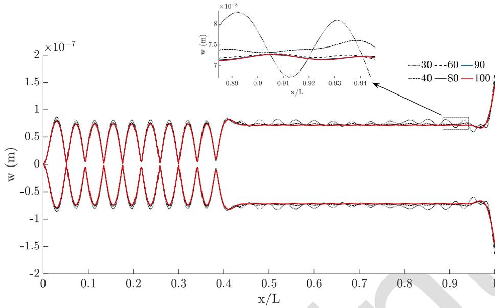
Figure 2. The TW response of a uniform beam using different numbers of trial functions.
