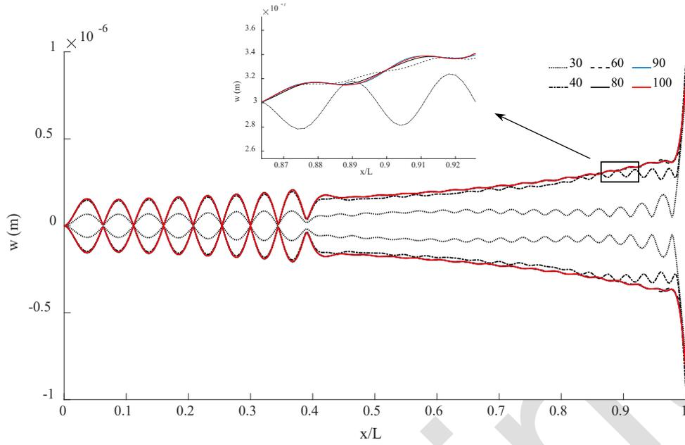
Figure 3. The TW response of the tapered beam using different numbers of trial functions.
