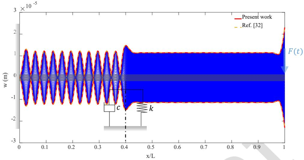
Figure 4. TW response comparison between the present study and [32]
