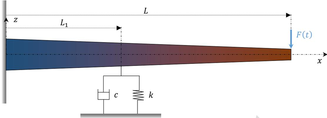
Figure 1. An Euler-Bernoulli cantilever non-uniform non-homogeneous beam with an intermediate passive absorber.
