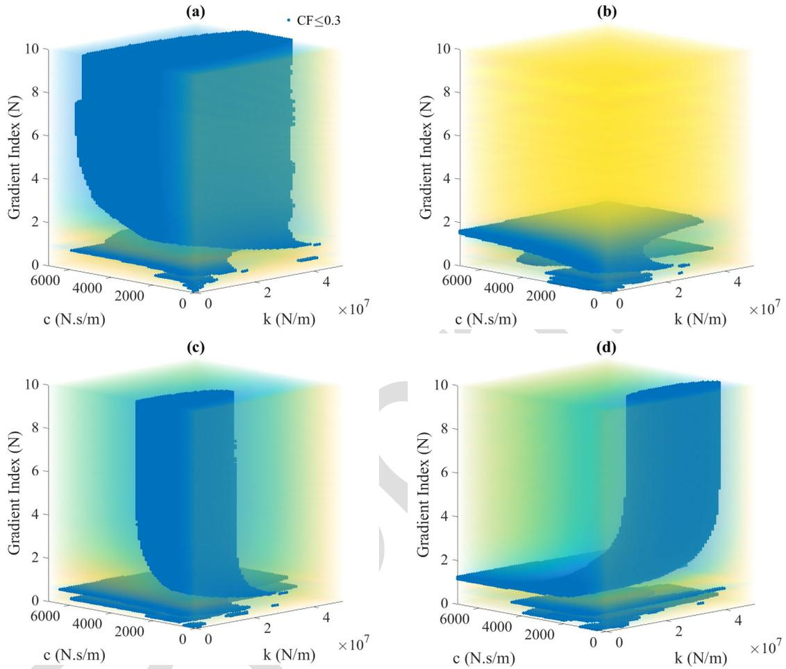
Figure 14. CF plots stack for varying  $N$  for (a) the tapered beam, (b) graded  $E$  and  $L_1 = 0.4L$ , (c) graded  $E$  and  $L_1 = 0.42L$ , and (d) graded  $\rho$ .
