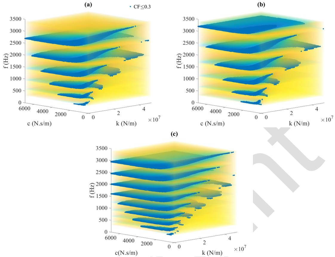
Figure 7. The stacked CF plots for the standard telephony range for (a) the tapered beam, (b) The beam where  $E$  is graded, and (c) The beam where  $\rho$  is graded.
