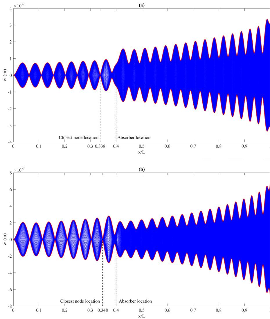
Figure 10. The displacement response of cross-sectionally tapered beams with (a)  $A(0)/A(L) = 6$  and (b)  $A(0)/A(L) = 12$  ratios
