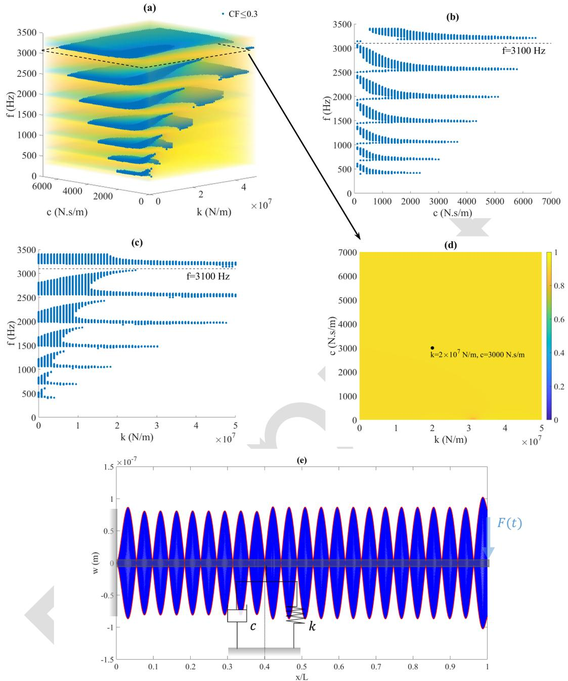
Figure 6. The stacked CF plots for the uniform homogeneous beam with marked below 0.3 values for the standard telephony range in (a) 3D view (b)  $f - c$  view (c)  $f - k$  view. (d) The CF plot for  $f = 3100$  Hz (e) The wave response of the beam with the absorber coefficients  $k = 2 \times 10^7$  N / m and  $c = 3000$  N. s / m.
