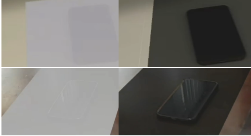
Fig. 6: Background and hologram color pairs. For optimal performance in obscuring physical objects, bright holograms on bright backgrounds are more effective than dark holograms on dark backgrounds.
