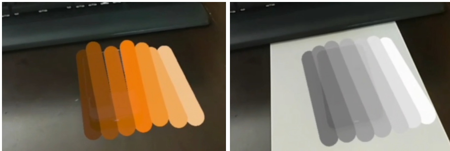
Fig. 5: Different colors of holograms. The intensity of the color brightness directly correlates with its ability to obscure objects behind it. Brighter colors render the background objects less transparent, which is critical.
