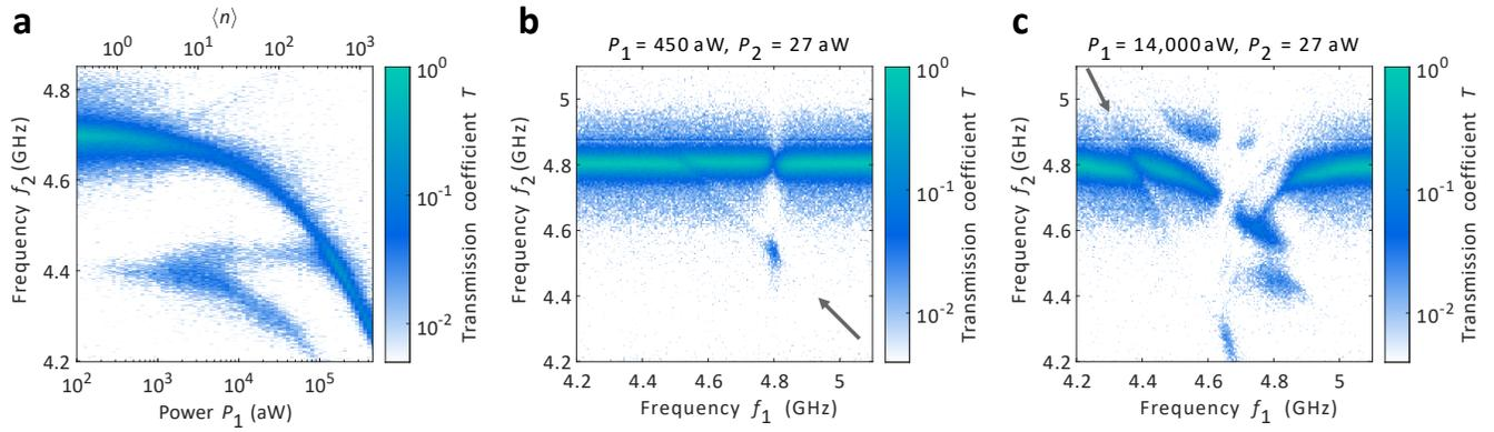
FIG. 3. **Strong drive response and photonic energy diagrams.** **a**, The two-tone measurement of Fig. 2d measured for two orders of magnitude stronger drive powers  $P_1$ . **b**, The second tone transmission coefficient  $T$  measured as a function of the two drive frequencies  $f_1$  and  $f_2$  at fixed  $P_1 = 450$  aW and  $P_2 = 27$  aW. **c**, The energy diagram measurement of Fig. 3b repeated for a stronger drive power of  $P_1 = 14,000$  aW.
