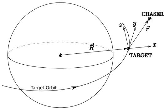
Fig. 1. Local-Vertical, Local-Horizontal (LVLH) frame.
