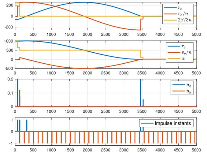
Fig. 3. Evolution in the original coordinates  $r_x, v_x/n$  together with the transformed state  $2\beta/3$  from (16) (top plot), as well as the original coordinates  $r_y, v_y/n$  together with the transformed state  $\alpha$  (second plot). Magnitude of the control input (third plot) and instants of impulses (bottom plot).
