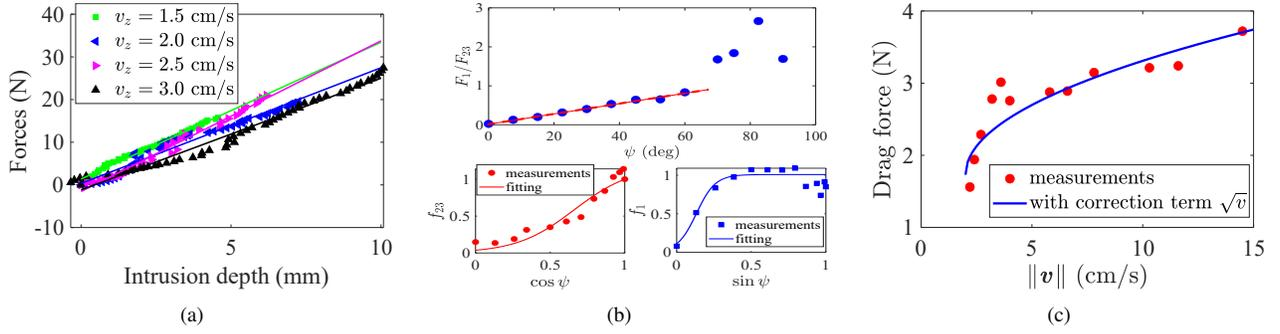
Fig. 4. Plate calibration results. (a) Vertical penetration resistive force versus intrusion depth. (b) Tangential and normal force relationship.  $f_1$  and  $f_{23}$  were fitted by sigmoid functions. (c) Horizontal penetration results under different velocities.
