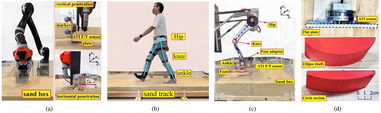
Fig. 3. The experimental setups. (a) RFT calibrations including vertical penetration tests for scale factor  $\zeta$  and horizontal penetration tests for  $f_1$  and  $f_{23}$ . (b) Humanoid walking gait capture using Vicon system. (c) Bipedal foot-terrain intrusions using a robotic leg. (d) Two selected non-flat foot models.
