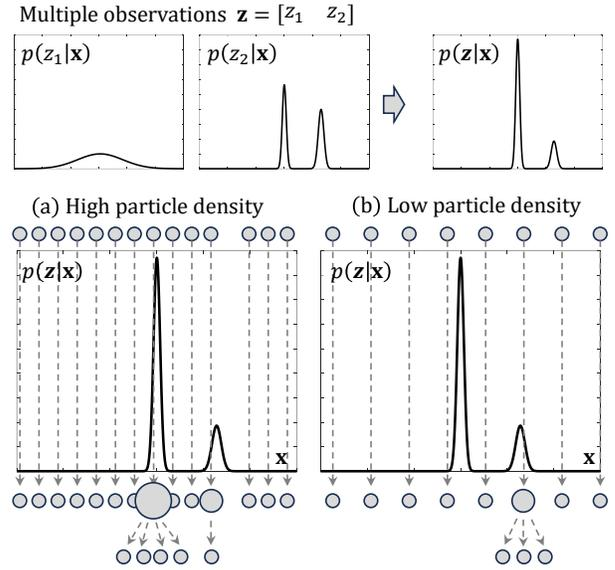
Fig. 1. Illustration of the normal particle filter (PF) in the presence of multiple observations with sharp peaks. When the initial particle distribution is widely spread and the number of particles is limited, the weights of particles at their true positions are not evaluated.
