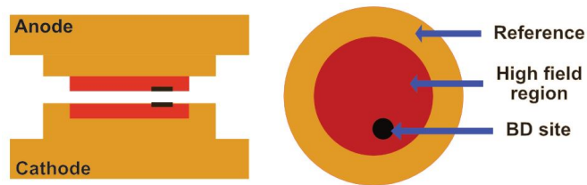
Figure 2: A schematic view of the electrodes under test. On the left: view from the side. On the right: top view, with a definition of different regions (valid for anode and cathode): reference - the region with no field (orange), high field region (red) and breakdown site (small black circle).
