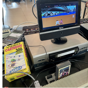
Figure 2: Turbo Soft's Videocartidge, unique Chilean interface from 1980s. Allowed using VHS video tapes as a high-capacity software storage for 8-bit Atari. Demonstration on Lost Party 2022.
