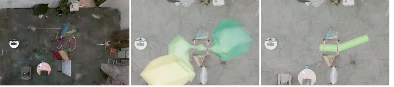
Fig. 3. Left: GSplat render of the scene. Middle: Generated safe polytope corridor colored with a gradient, with each successive polytope being a slightly different color. The corridor is visualized in a “meshed” version of the ellipsoids from GSplat. Right: Finite horizon planned path (inflated to represent geometry of agent) through the corridor.
