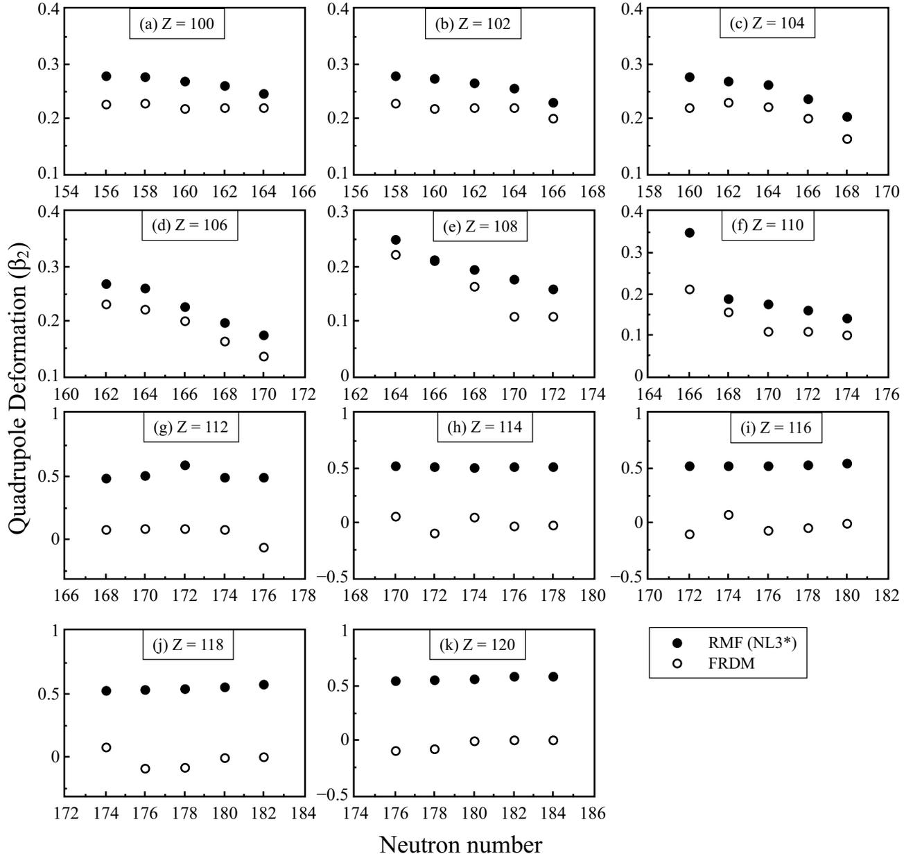
FIG. 2. (Color online) The quadrupole deformation parameter ( $\beta_2$ ) for the isotopic chain of  $Z = 100$  to  $120$  nuclei by using relativistic mean-field approach with NL3\* are given along with the FRDM predictions [75, 76].
