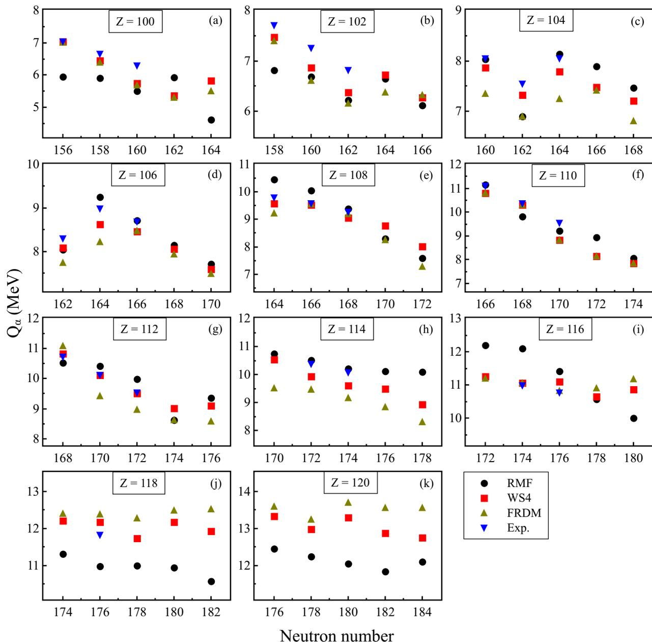
FIG. 1. (Color online) The  $\alpha$ -decay energy for the isotopic chain of  $Z = 100$  to 120 is calculated via RMF (NL3\*) and compared to the FRDM results, [72] WS4 predictions, [73] and the existing experimental data.[74]
