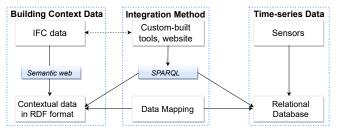
Fig. 6 Semantic + Relational Database BIM-IoT integration method (Adapted from [66]).
