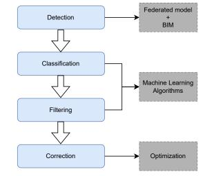
Fig. 8 Clash management process and enabling methodology
