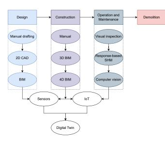
Fig. 2 Civil engineering phases and evolution of enabling technologies
