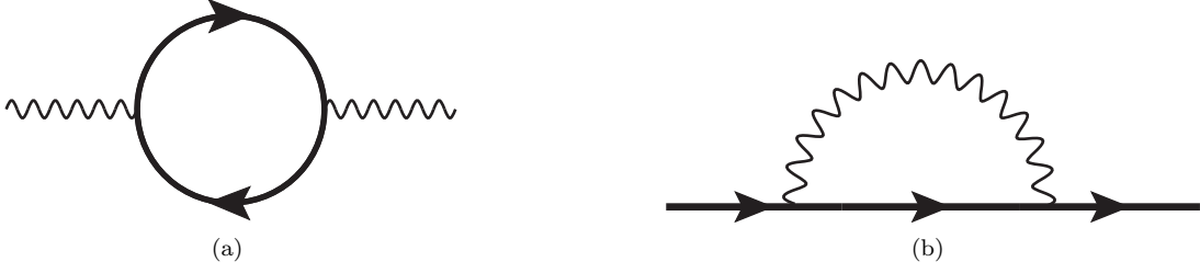
FIG. 2. The one-loop diagrams for (a) the boson self-energy and (b) the fermion self-energy. Curves with arrows represent the bare fermion propagator G_{(0)} , whereas the wiggly lines represent the dressed bosonic propagator D_{(1)} .
