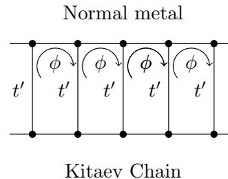
FIG. 1. Schematic diagram of a Kitaev chain side-coupled to a normal metal.  $t'$  is the hopping amplitude between the two chains.  $\phi$  quantifies the magnetic flux piercing through each plaquette.
